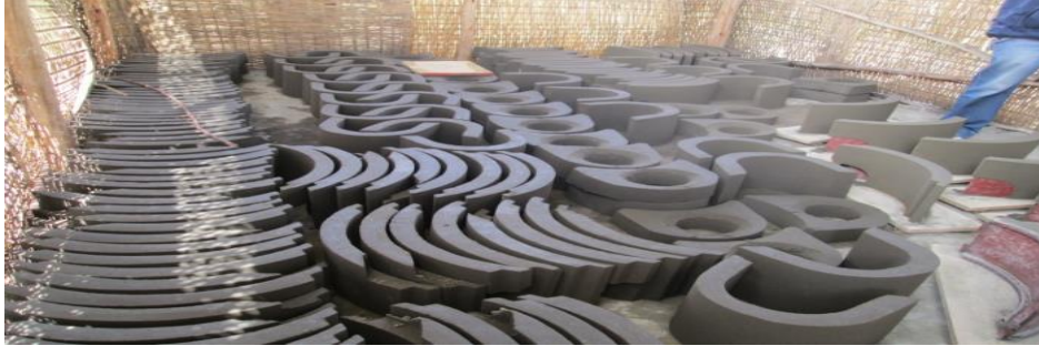
Fig 3: Parts of Fuel saving stoves
